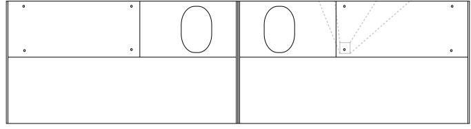
If for some reason the sliding bookcases do not roll smoothly or seem to not be level, you can easily adjust the bookcases by tightening or loosening the adjustment bolts located at the bottom. To adjust the bookcase higher, loosen the bolt/ bolts and to lower the bookcase tighten the bolt/ bolts.
