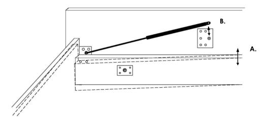
**Step 10:**Repeat Step 8-9 to install second Air Piston on left side of bed.
